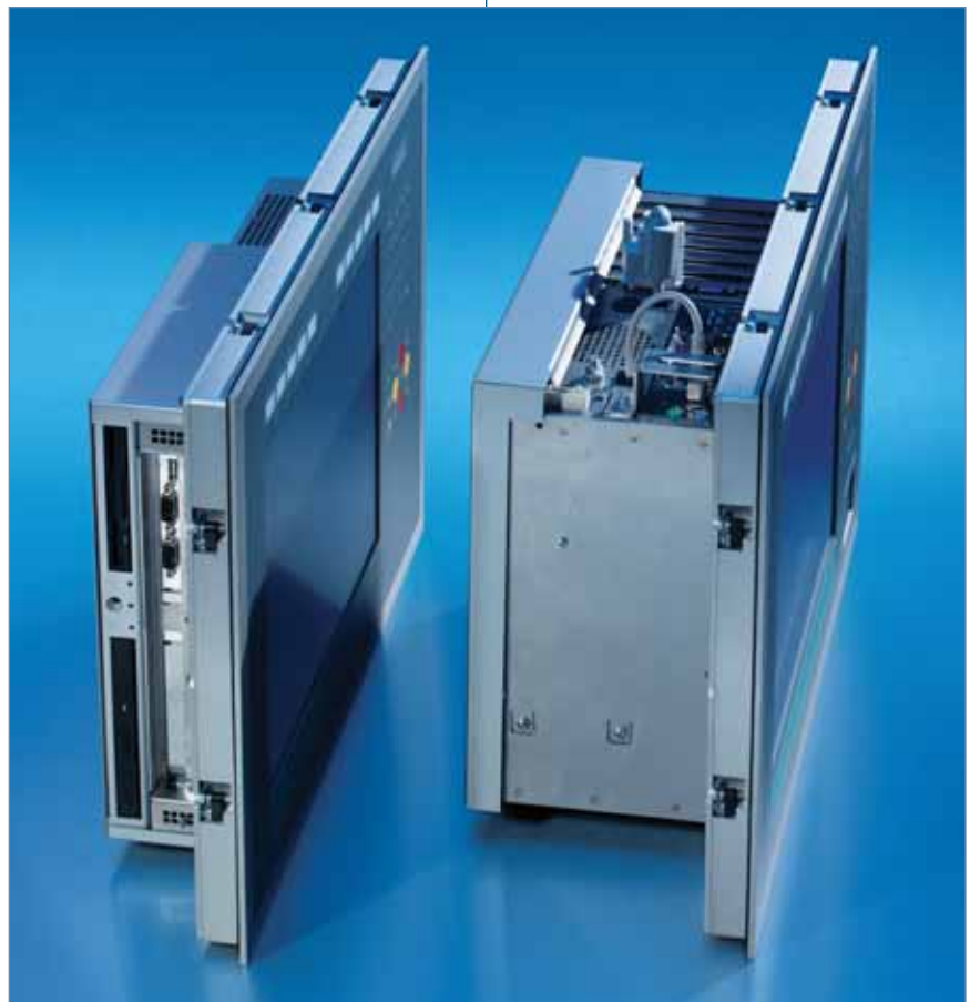
Beckhoff's Panel PCs integrate LCD monitors from 6.5 to 20 in. with PCs.
