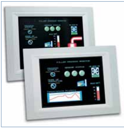
IDEC's HG3F and HG4F are 256 color TFT LCD screens with 10.4 and 12.1 in. screens (respectively).
